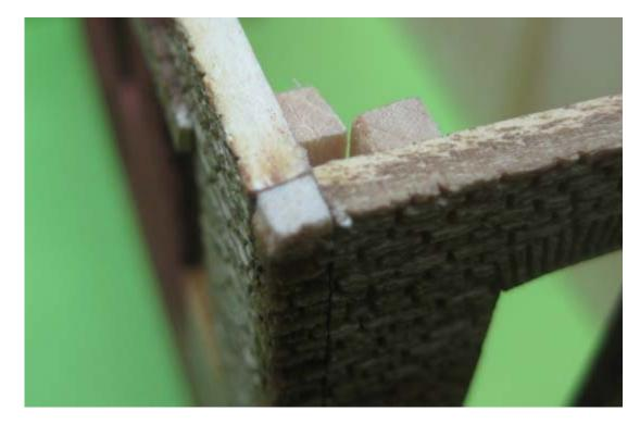
Once your Corner Pieces are installed and dry, you may need to scratch up the joint lines between the bricks. Not too much...
