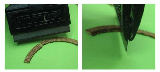
Use a "chopping" motion to cut straight through the mortar line. Once you have one Lintel cut, line it up to make sure it fits your window properly.
